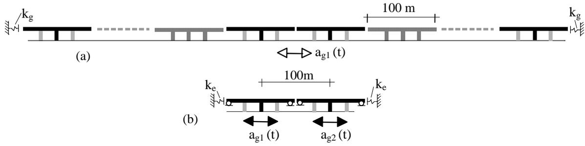
Figure 2(a) and (b). Bridge structures. (a) Multi-span model, and (b) two-span model
