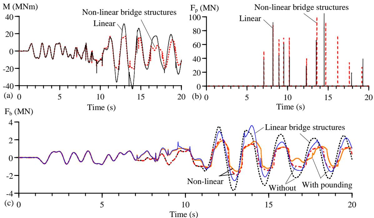
**Figure 6(a)-(c).** Influence of non-linear material properties on (a) bending moment  $M$  at the left pier support, (b) contact force  $F_p$  between the girders, and (c) bearing force  $F_b$
