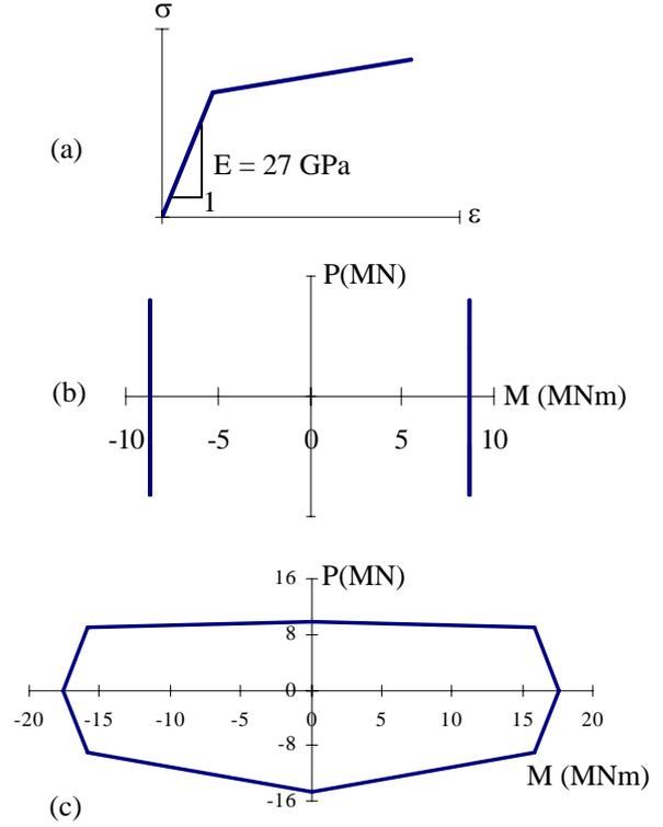
Figure 3(a)-(c). RC pier and girder material properties. (a) Stress-strain relationship, (b) girder yielding surface, and (c) pier yielding surface
