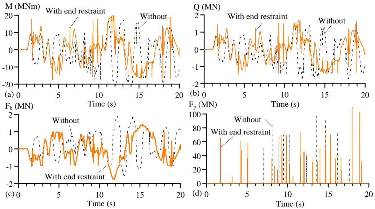
**Figure 7(a)-(d).** Influence of the end restraints on the activated forces. (a) Bending moment  $M$ , (b) shear force  $Q$  at the left pier support, (c) bearing force  $F_b$  at the left pier top, and (d) contact force  $F_p$  between the girders.
