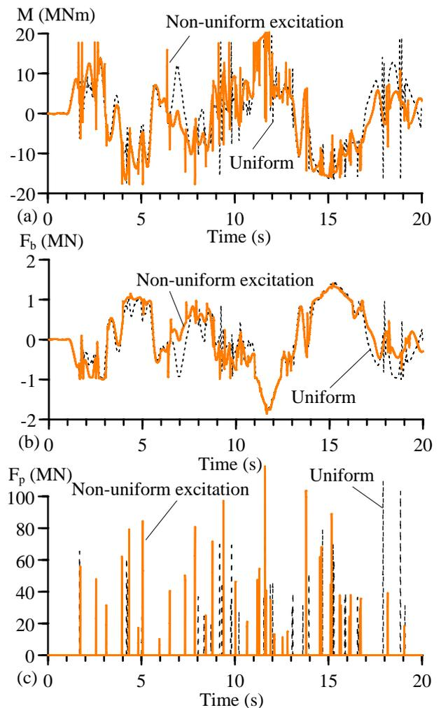
**Figure 8(a)-(c).** Effect of non-uniform ground excitation on activated force. (a) Bending moment  $M$  at the left pier support, (b) bearing force  $F_b$  at the left pier top, and (c) contact force  $F_p$  between the girders.
