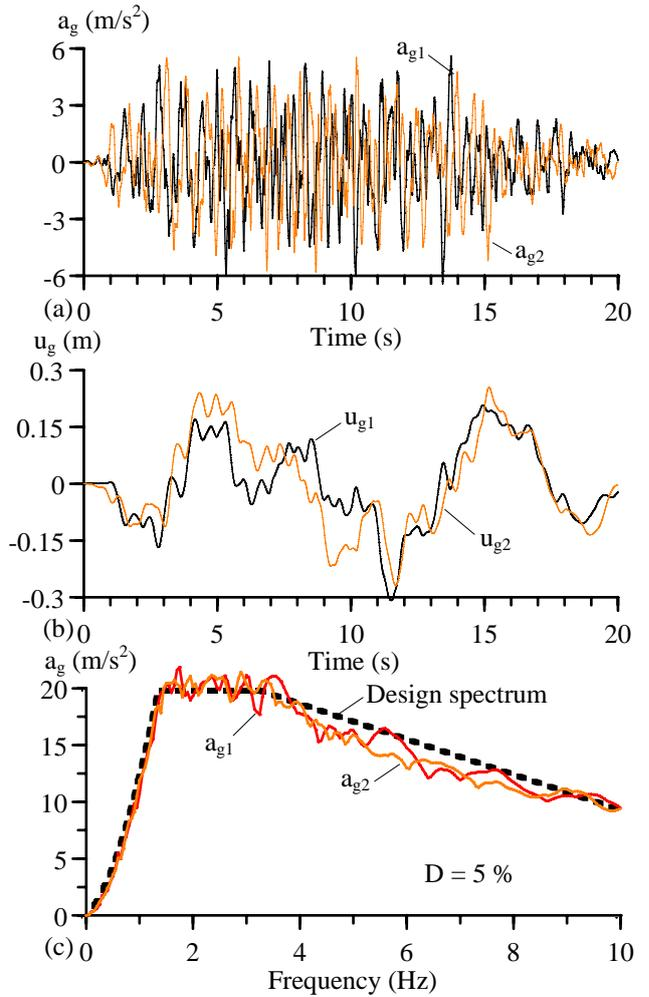
**Figure 1(a)-(c).** Non-uniform ground motions. (a) Ground accelerations  $a_g(t)$ , (b) ground displacements  $u_g(t)$ , and (c) corresponding response spectra with the Japanese design spectrum for hard-soil site.
