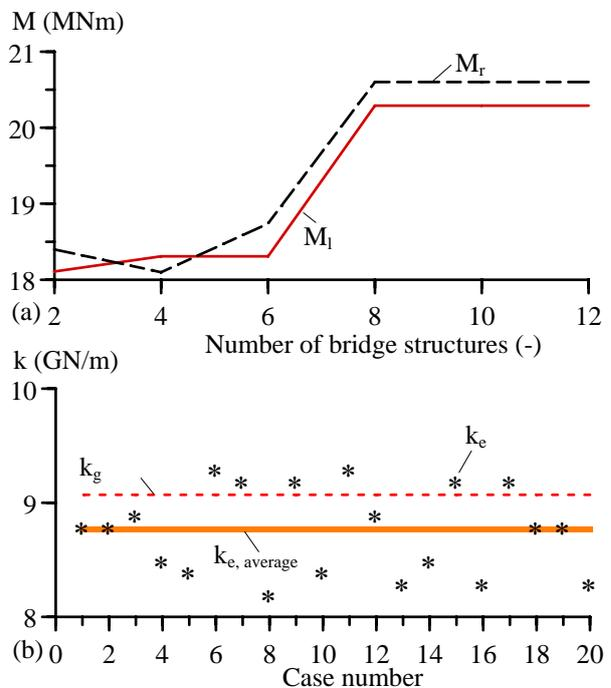
**Figure 5(a) and (b).** Effect of the number of the considered bridge structures on (a) the bending moment  $M$  development, and (b) development of the end-restraint stiffness with the considered cases.
