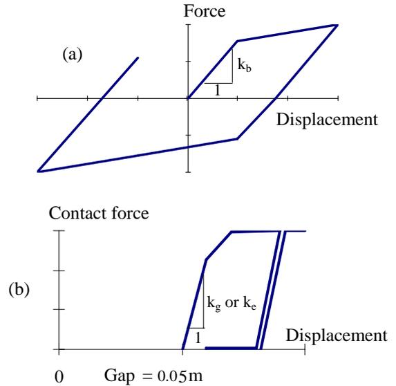
Figure 4(a) and (b). Bearing and impact element stiffness model. (a) Bearing and (b) impact element
