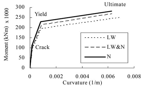
**Figure 6.** Arch springing skeleton curve
