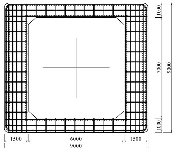
Figure 4. Reinforcement of lower pier (unit mm)
