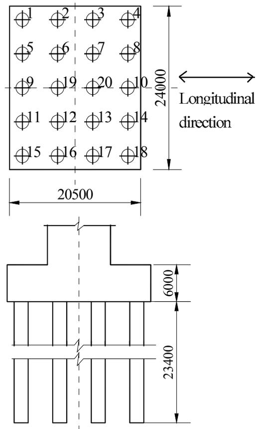
**Figure 9.** Piles arrangement
