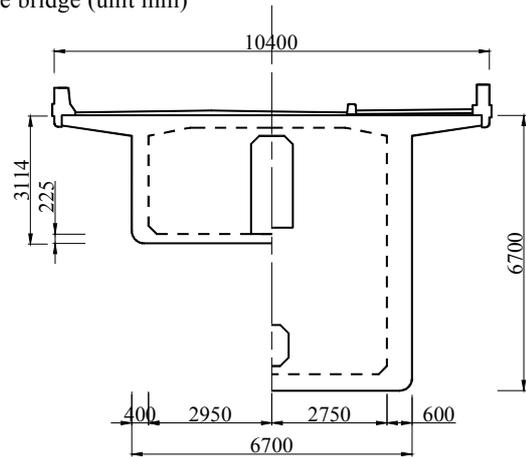
Figure 2. Cross section of girder (unit mm)
