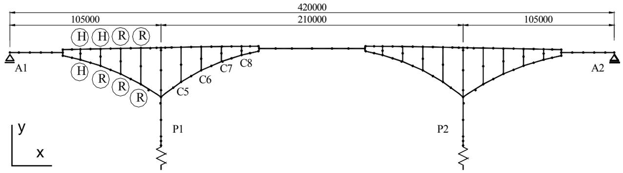
Figure 5. Analytical model (longitudinal direction) (unit mm)
