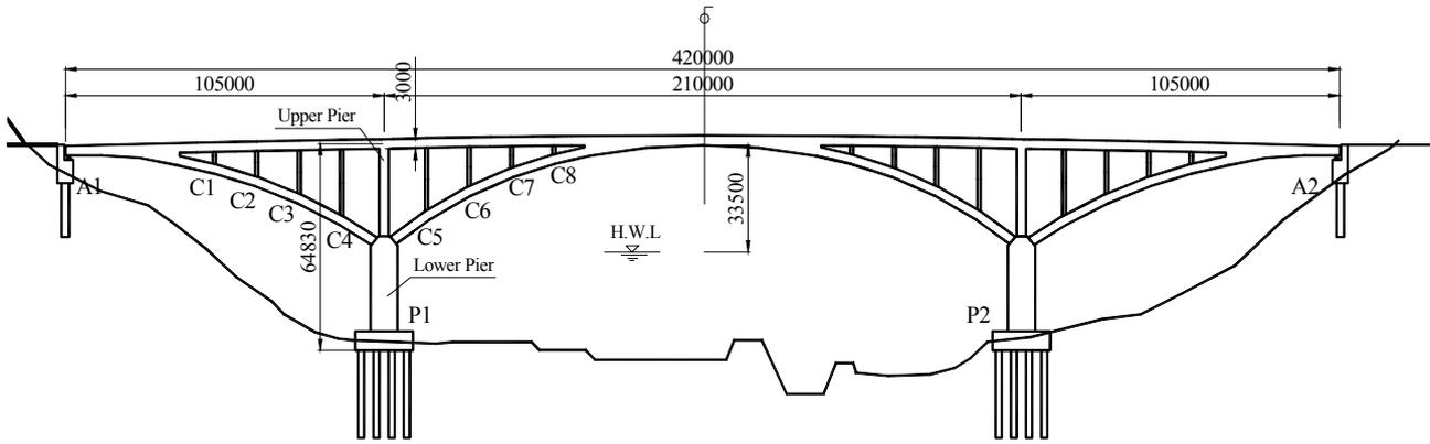
Figure 1. Elevation view of the bridge (unit mm)
