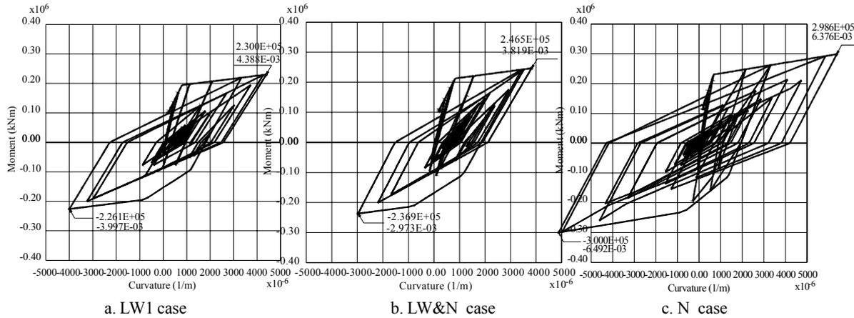
Figure 8. Response M- of the arch springing section (longitudinal direction)
