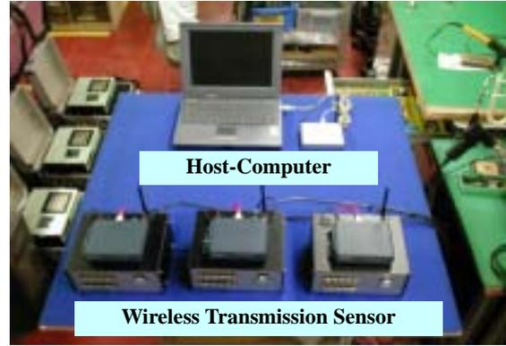
Figure 1. Wireless data acquisition
