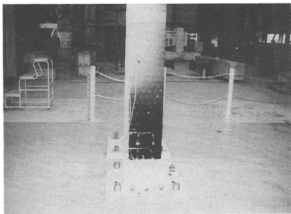
Fig. 6 Upright cantilever on a shaking table
