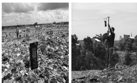
Fig. 4. Measurement of ambient methane concentration by pole method.
