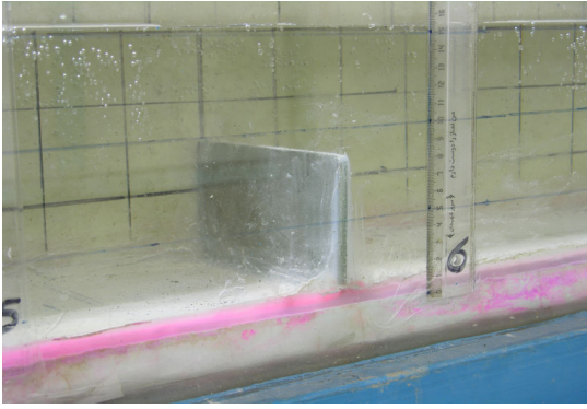
Fig. 2 A photograph of installed baffle
