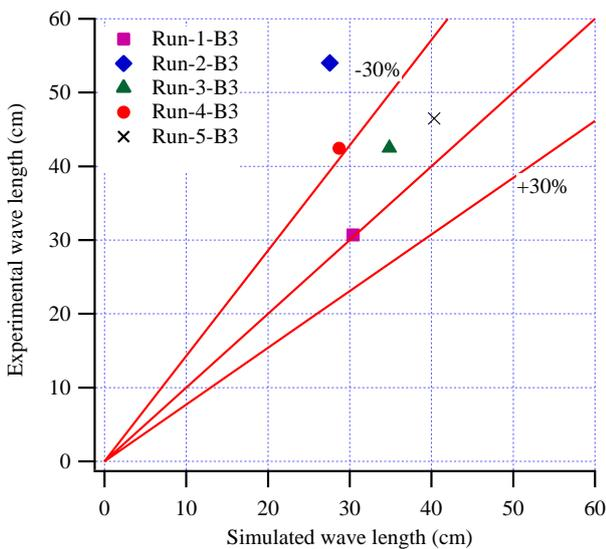
b. The comparison between the experimental results and the simulated results of the wave length of sand dunes.
