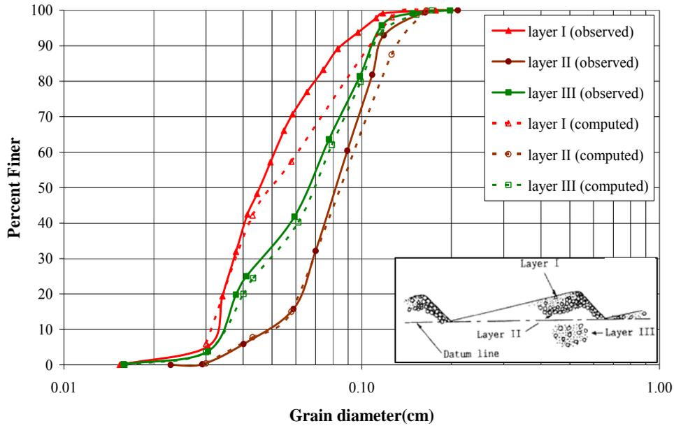
a. The comparison of grain size distributions (Run-2-B3) where the locations of measured mixture are shown as a small figure.
