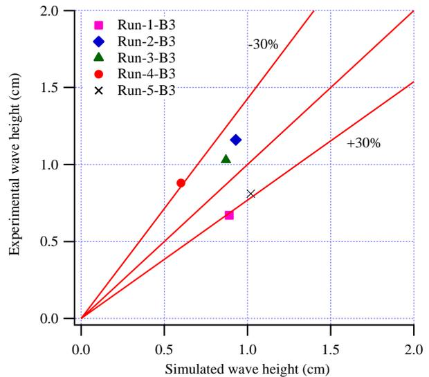
c. The comparison between the experimental results and the simulated results of the wave height of sand dunes.
