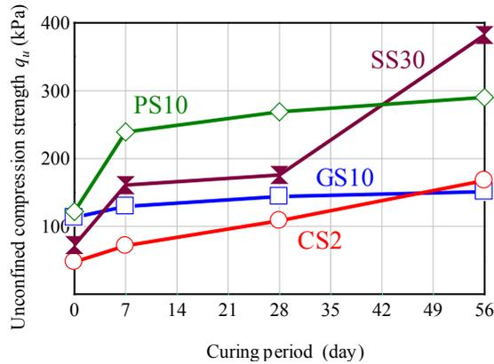
**Fig. 6** The effect of curing period on unconfined strength
