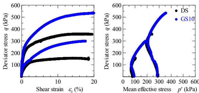
Fig. 10 Undrained triaxial test results of GS10
