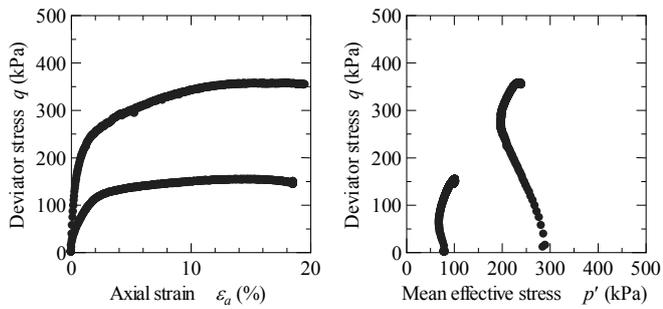
Fig. 8 Undrained triaxial test result on the dredged soil
