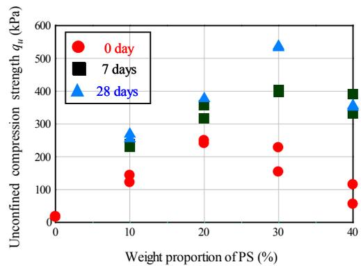
**Fig. 5** Unconfined compression test results of the treated soils with different weight proportions of stabilizers
