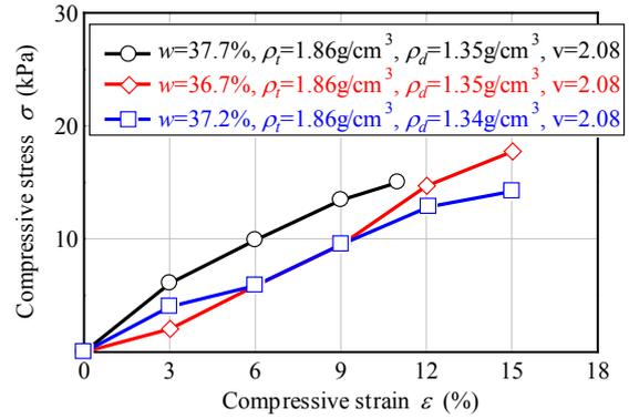
**Fig. 3**  $\sigma - \varepsilon$  curve in unconfined compression test of DS**Table 2** Main compositions of stabilizers
