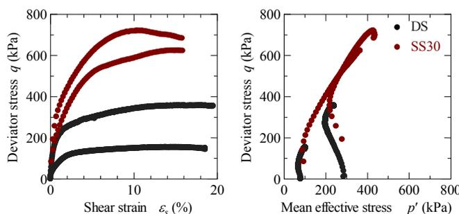
Fig. 11 Undrained triaxial test results of SS30
