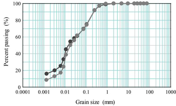
**Fig. 1** Grain size distribution of DS
