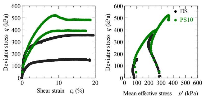
Fig. 12 Undrained triaxial test results of PS10
