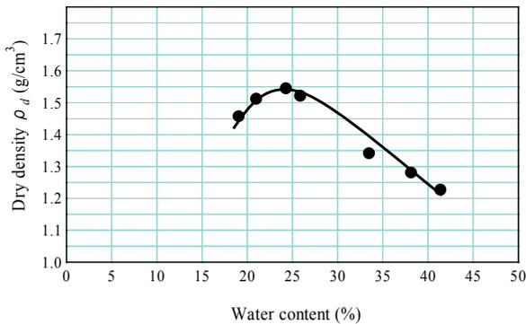
**Fig. 2** Compaction curve of DS
