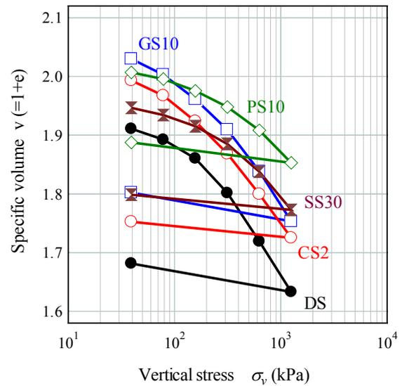
**Fig. 7** Oedometer test results
