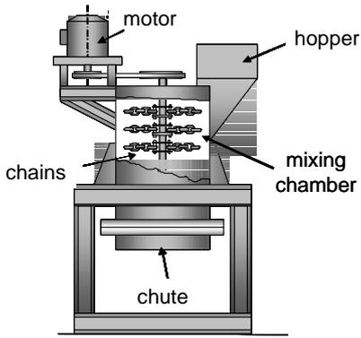
**Fig. 4** Chain rotary crusher-mixer<sup>1)</sup>
