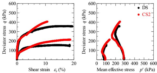
Fig. 9 Undrained triaxial test results of CS2
