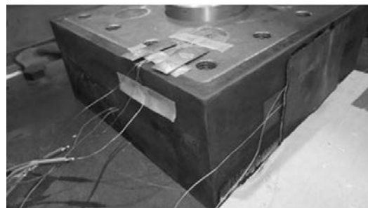
Figure 5. Thermocouples installed on the specimen
