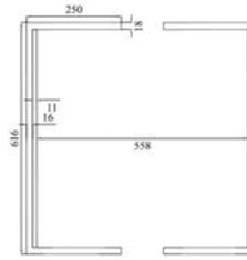
**Fig.10.** Detailed cross section of improved diagonal members to increase traffic capacity (Dimensions in mm)
