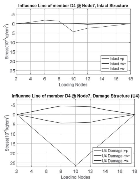
**Fig.4** Influence lines of member D4 at node 7 for intact and damage structures (U4 damage)
