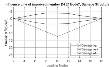
**Fig.9.** Influence lines of member D4 at node 7 for improved damage structure for minimum requirement
