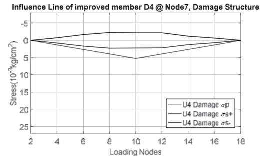
**Fig.11.** Influence lines of member D4 at node 7 for improved damage structure to increase traffic capacity
