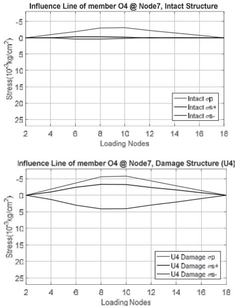
**Fig.5.** Influence lines of member O4 at node 7 for intact and damage structures (U4 damage)
