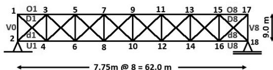
Fig.1 Double diagonal single span truss bridge
