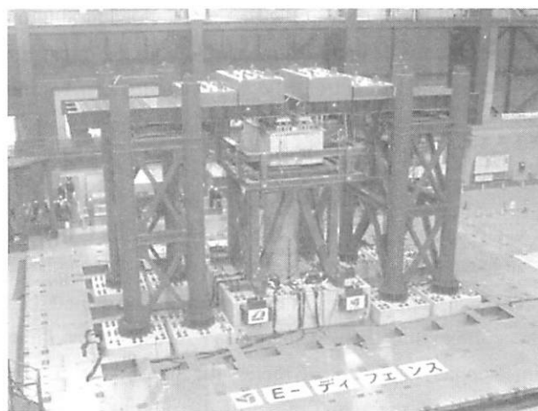
Fig. 1 Shake Table Test Using E-Defense
