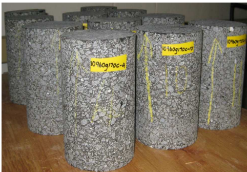
Fig.1 100mm x 150mm cylindrical test specimens.
