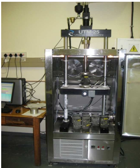
Fig.2 Dynamic modulus setup with IPC UTM-25.
