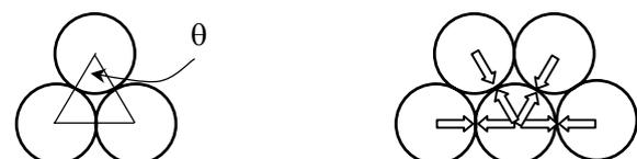
**Fig.2** Illustrations of microstructure of the doublets and the micro stresses (2005)
