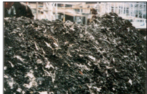
Figure 20 Milled pavement containing sheeting fragment
