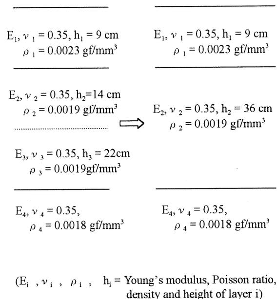
**Fig.7** Pavement structure of Road Test Section 609
