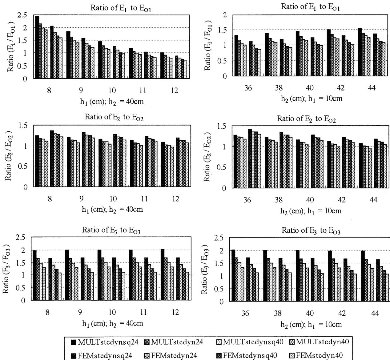
**Fig.6** Backcalculated layer moduli using MULTstc and FEMstc on peak dynamic deflections
