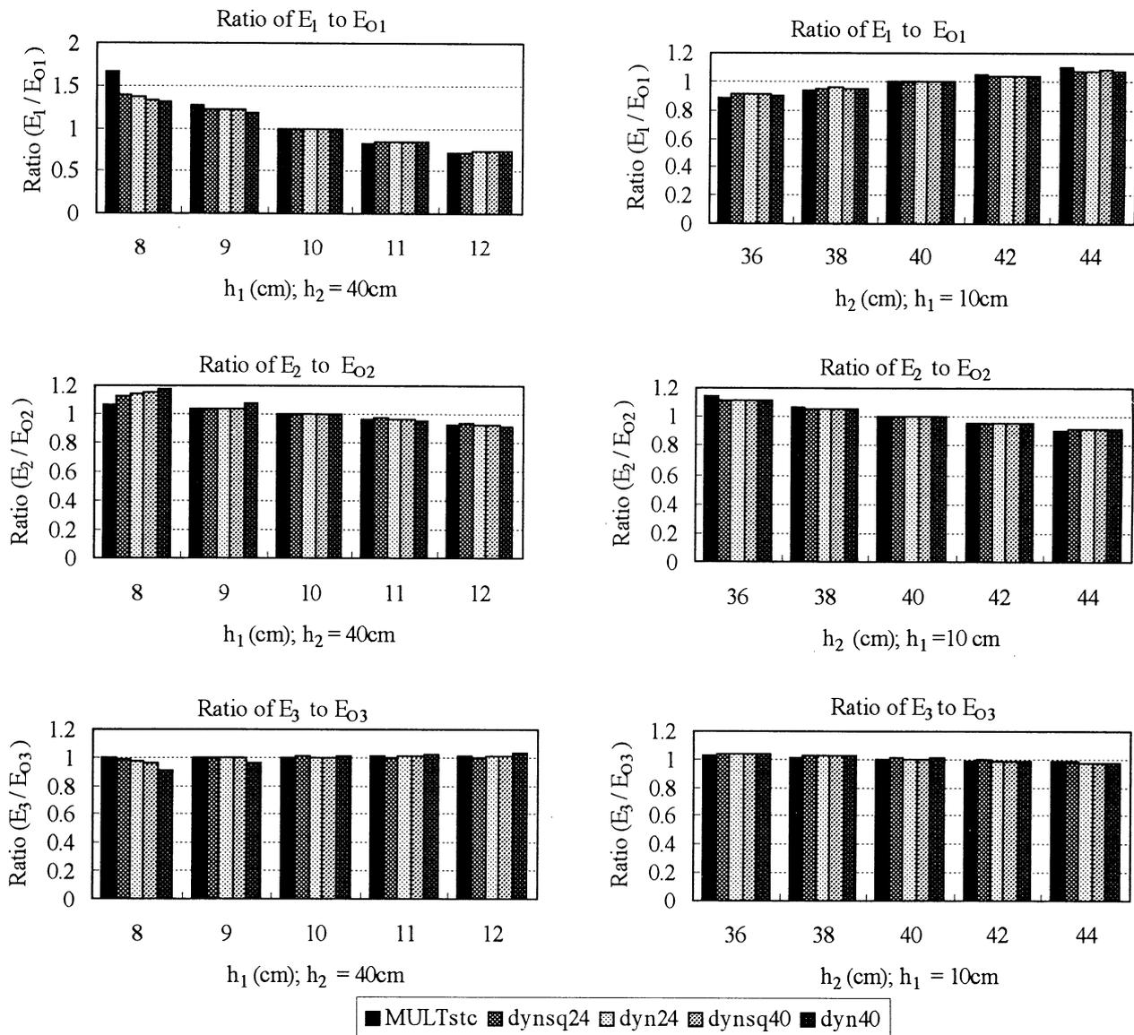
Fig.4 Effect of errors in  $h_1$  and  $h_2$  on backcalculated layer moduli for the hypothetical pavement model
