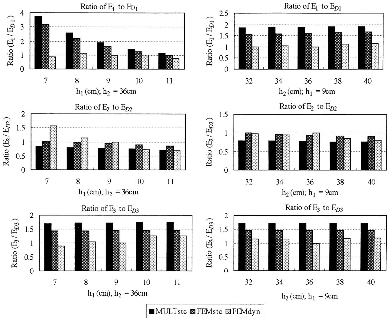
Fig. 8 Backcalculated layer moduli for Section 609
