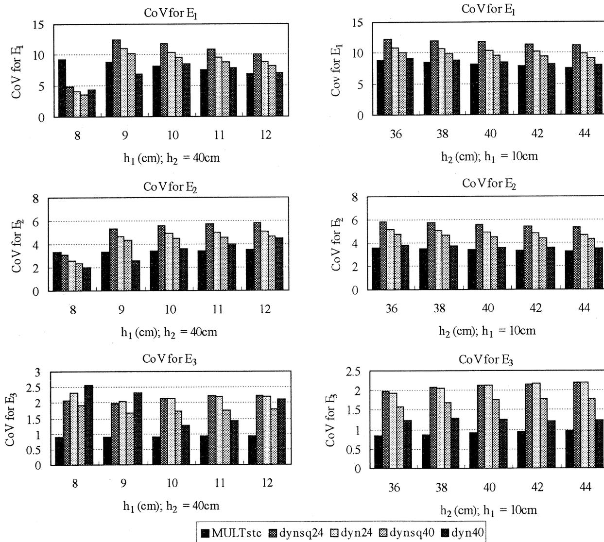
Fig. 5 Coefficient of Variation (CoV) for the backcalculated layer moduli
