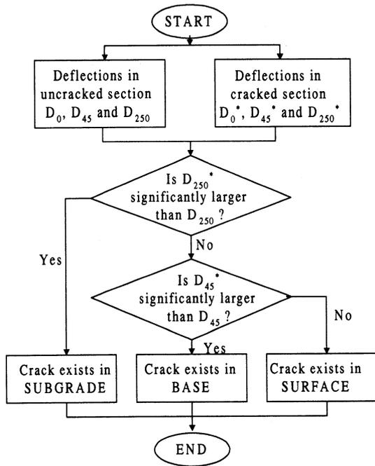
Fig. 6 Flow chart for evaluating the seriousness of crack
