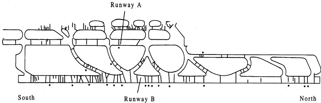
Fig. 1 Earthquake induced cracks in runways of Osaka International Airport
