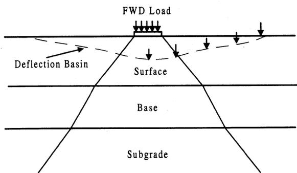
Fig. 3 Distribution of vertical strain under FWD loading
