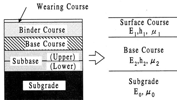
Fig. 4. Pavement structure model for theoretical analysis
