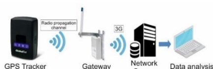
Figure 1: Scheme of radio wave propagation experiment
