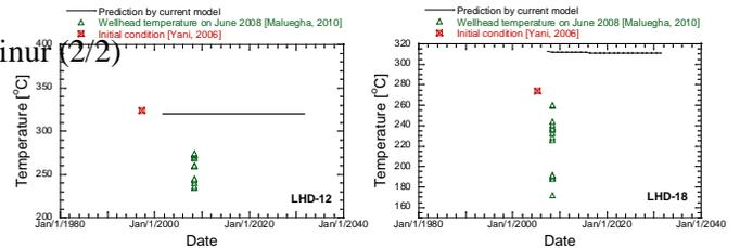
**Figure 3:** Comparison of evolution temperature between measurements and predictions.
