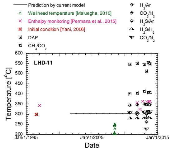
**Figure 4:** Comparison of evolution temperature in LHD-11 among initial condition, wellhead temperature, enthalpy monitoring, gas geothermometer data, and predictions.
