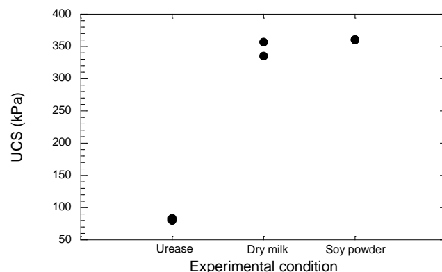
Figure 4. The relation between the UCS test with various treatment solution
