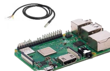
Fig. 1.0 DS18B20 Temperature Sensor and the Raspberry-Pi Micro-controller
