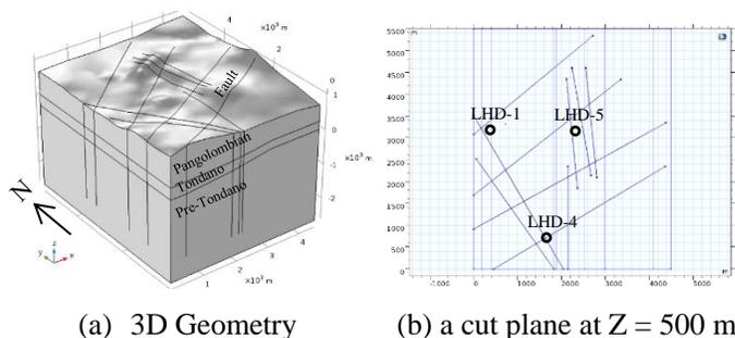
**Figure 2:** Model geometry in COMSOL Multiphysics
