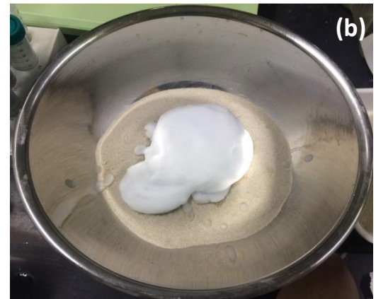
Figure 1. (a) Precipitation in centrifuge tube, (b) hard gel being mixed with sand
