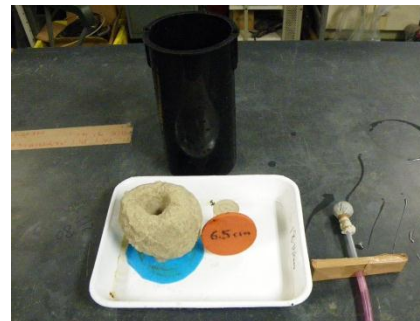
Fig.4. Improved sand sample with mid-cylinder arrangement
