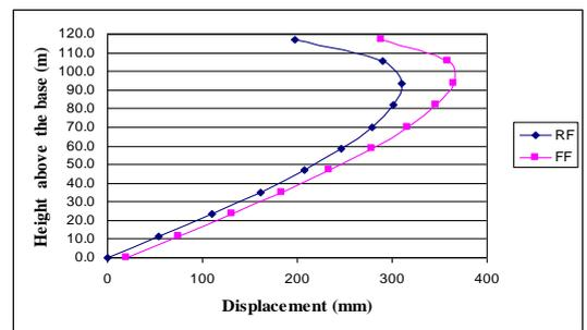
Fig.3: Vertical displacement profile along a vertical through the centre of core
