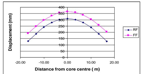
Fig.4: Vertical displacement profile along a horizontal through maximum displacement
