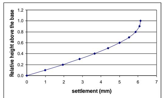
Fig.5: Displacement profile for homogeneous embankment
