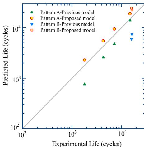
Fig. 2. Comparison of predicted and experimental lives for Inconel 718.
