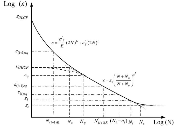
Fig. 1. Proposed strain-life curve.
