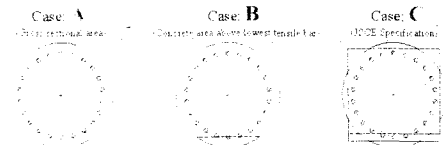
Fig.2 Parameter for effective concrete area
