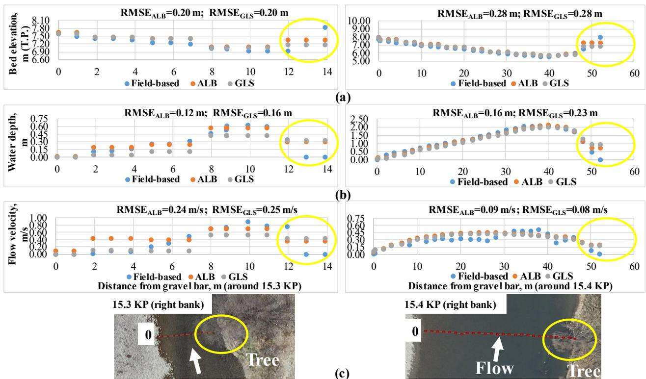
**Fig.3** Comparison of field-observed (a) bed elevation, (b) water depth, and (c) flow velocity with respective simulated values at a low discharge of  $26.16 \text{ m}^3/\text{s}$ , using ALB and GLS data along the two surveyed local cross-sections
