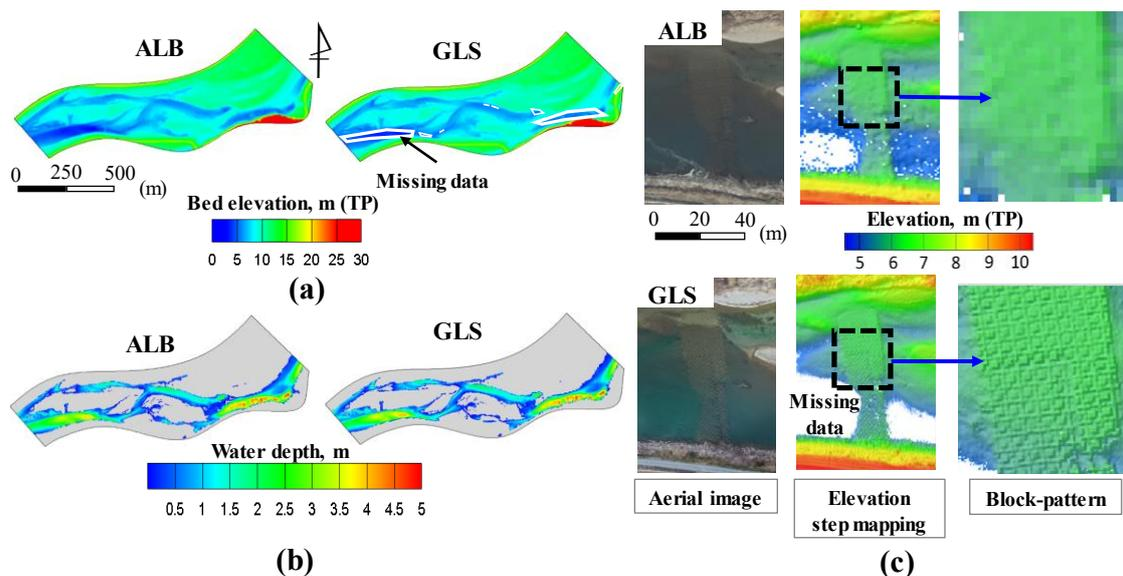
Fig.2 (a) Bed elevation, (b) numerically simulated water depth mapping, and (c) reproducibility of submerged infrastructure; herein, Tokyo Peil (TP) denotes the average sea level in Tokyo Bay, Japan
