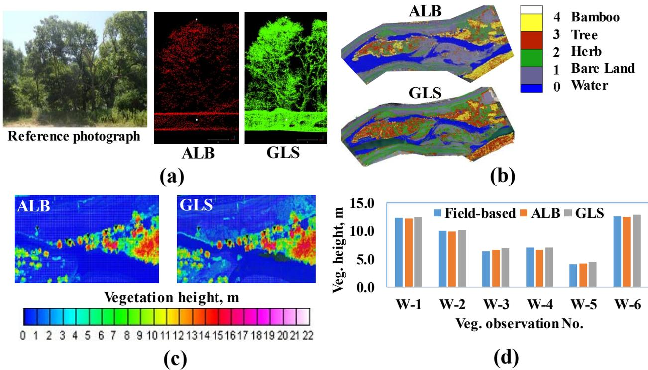
**Fig.4** (a) Vertical structure, (b) land cover mapping, (c) vegetation height contour map, and (d) comparison of ground-surveyed woody vegetation heights with ALB and GLS data estimates
