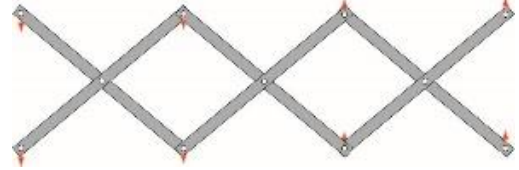
Fig. 3 Primary vibration mode (SE)
