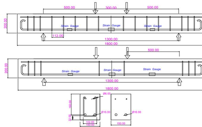
Figure 1. Dimension and loading of RC beams
