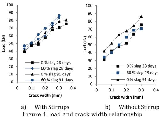
Figure 4. load and crack width relationship
