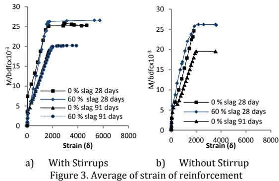
Figure 3. Average of strain of reinforcement
