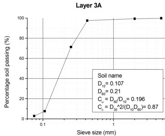
Fig.4 Size particle of layer 3A
