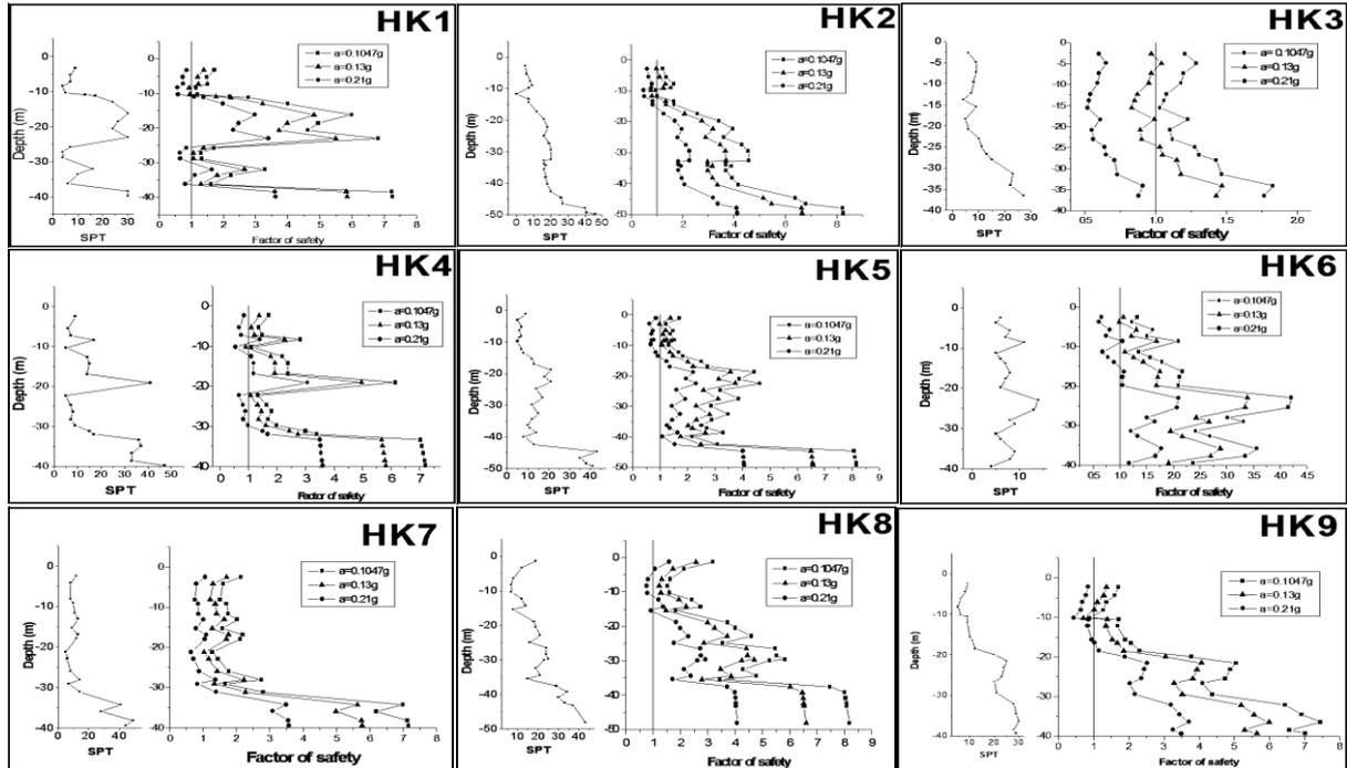
Fig.3 Factors of safety against liquefaction at boreholes HK1 to HK9.
