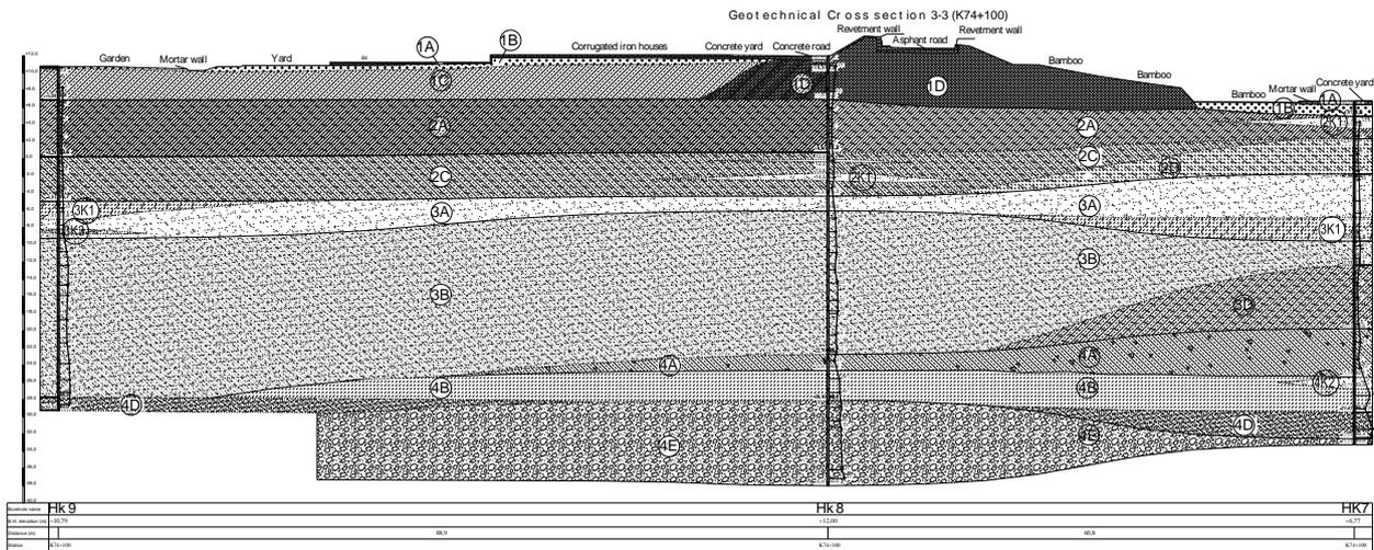
**Fig.2** Geotechnical cross section 3-3 (K74+100).
