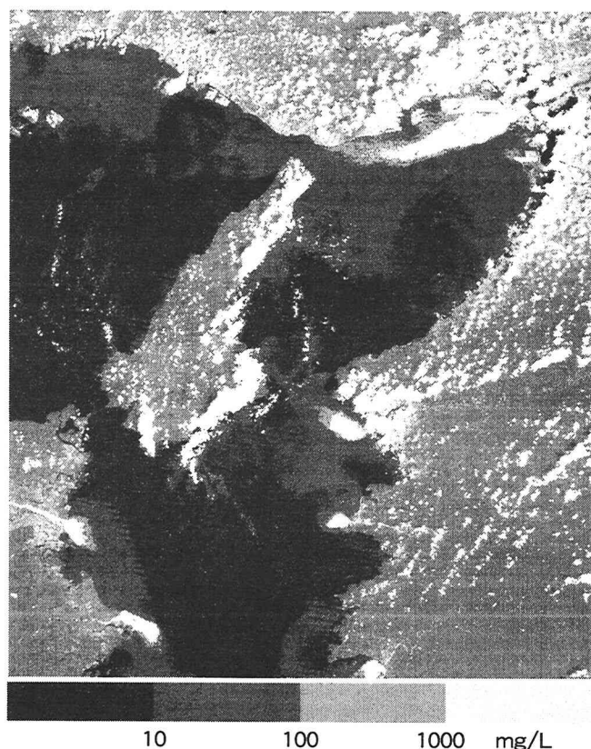
Fig.8 Contour of soil particle concentration around Osaka bay at 1989.9.4
