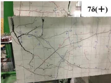
図-5 損傷状況 (No. 1)
