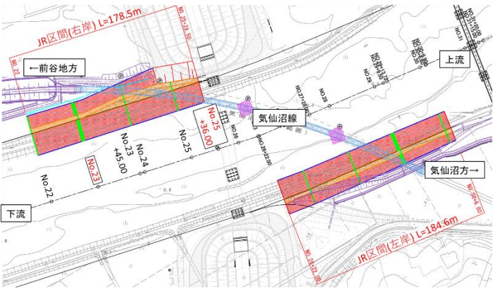
図-1 築堤護岸工事施工範囲
