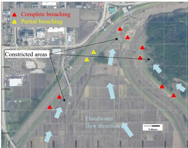
Figure 1. Complete and partial breaching locations of river embankment in Marumori area, Miyagi
