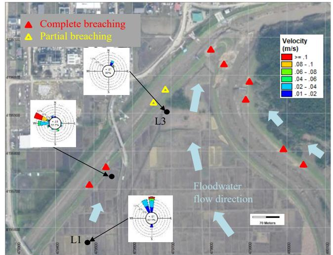
Figure 5. Flow velocity and direction
