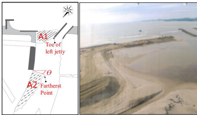
Figure 3: Left: Definition of river mouth quantities, Right: Artificial sandspit (2018/03/19)
