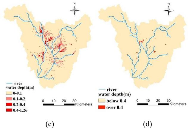
Fig.5 (c) simulated flood in 1993 (d) inundation over 40cm in 1993
