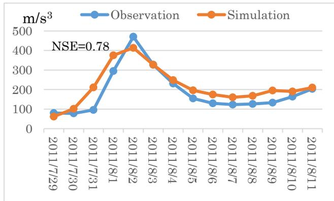
Fig.3 the simulated and observed discharge at P1 gauge
