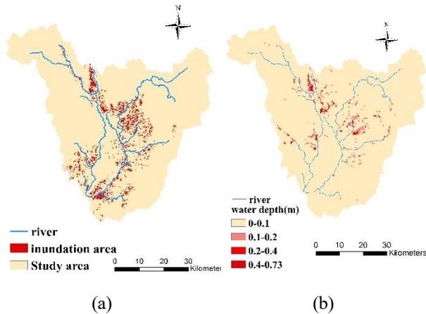
Fig.4 (a) the satellite recorded inundation area in Aug 5th, 2011; (b) simulated inundation area of Aug 2011
