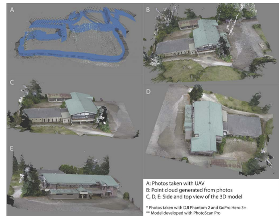
Figure 2: 3D model of a house using UAV imagery
