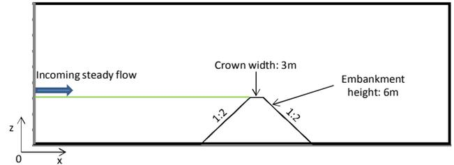
Figure 1. Domain sketch for numerical model
