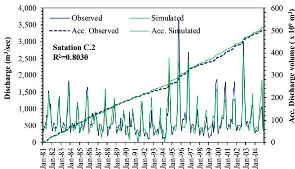
Fig. 3 Comparison on river discharge for C.2 gaging station
