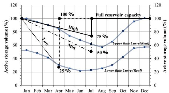
Fig. 2 A simplified upper reservoir operation rule curve
