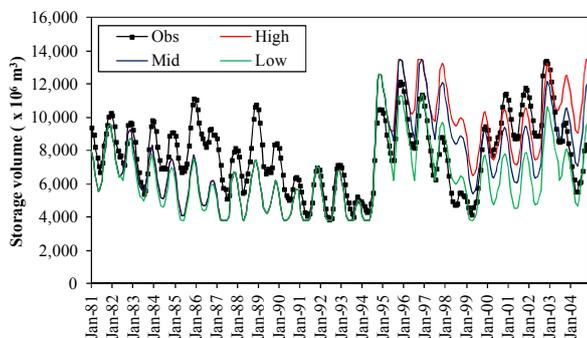
Fig. 4 Simulated of storage volume for Bhumibol reservoir
