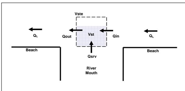
Fig.1 Definition sketch for simulating sand terrace
