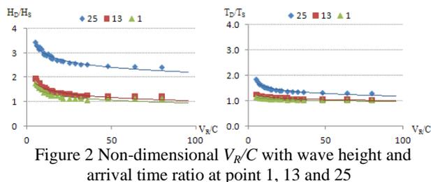
Figure 2 Non-dimensional  $V_R/C$  with wave height and arrival time ratio at point 1, 13 and 25
