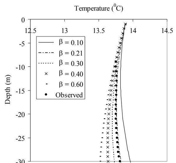
**Fig. 1** Simulated temperature-depth profiles at W4
