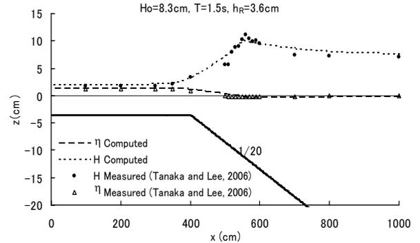
Fig. 1 Measured and calculated wave height and wave set-up at a river mouth
