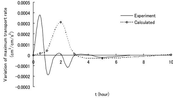
**Fig. 2** Variation of maximum sediment transport rate at the river mouth, Case  $h_R=1\text{cm}$ ,  $H_0=6\text{cm}$ ,  $T=1.44\text{s}$ , slope  $i=1/10$
