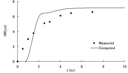
**Fig. 3** Development of sand bar height Case  $h_R=1\text{cm}$ ,  $H_0=6\text{cm}$ ,  $T=1.44\text{s}$ , slope  $i=1/10$
