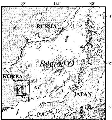
Figure 1. Nested grid system for the tsunami numerical model in the Japan (East) Sea.
