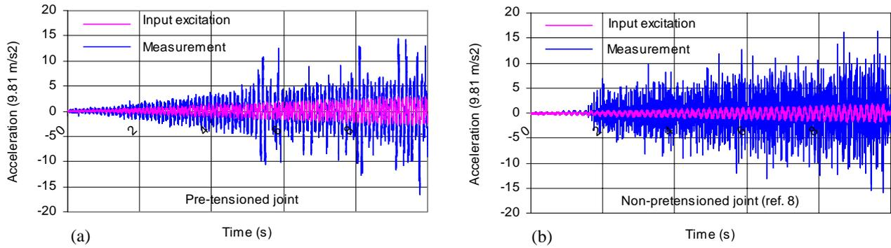
Fig.6 Time-histories acceleration at the top of the test columns: (a) Pre-tensioned joint; and (b) Non-pretensioned joint (ref. 8)
