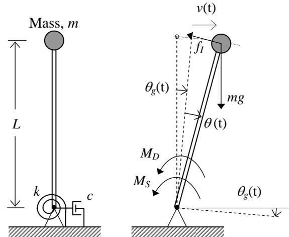
Fig.2 Mechanical model and its free-body diagram due to ground-induced motion
