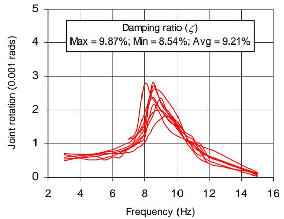
Fig.5 Frequency-response curve of the pre-tensioned joints
