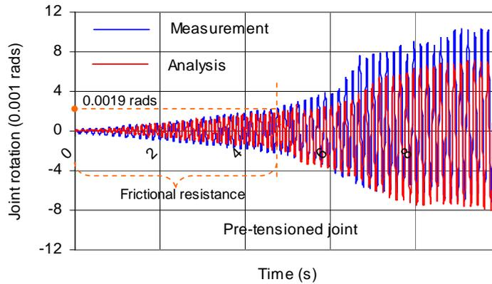
Fig.7 Time-history joint rotation of the pre-tensioned joint
