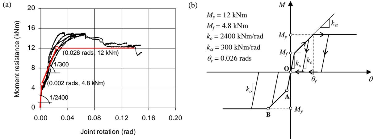
Fig.3 Moment rotation curve of pre-tensioned joint: (a) Experimental curve (ref. 3); and (b) Hysteretic model
