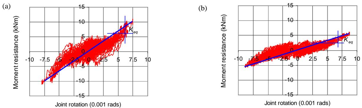
Fig.8 Predicted time-history moment rotation: (a) Pre-tensioned joint; and (b) Non-pretensioned joint (ref. 8)
