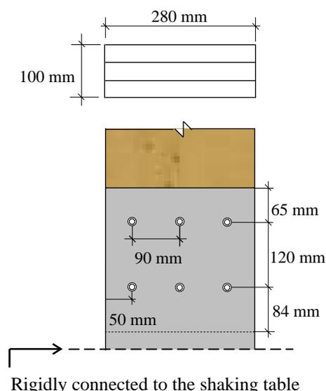
Fig.1 Geometry of moment-resisting joint
