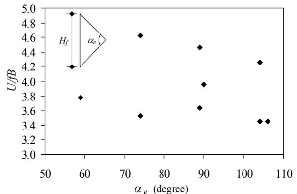
Figure 5(c) Flutter speed v.s. Angle of fairing tip
