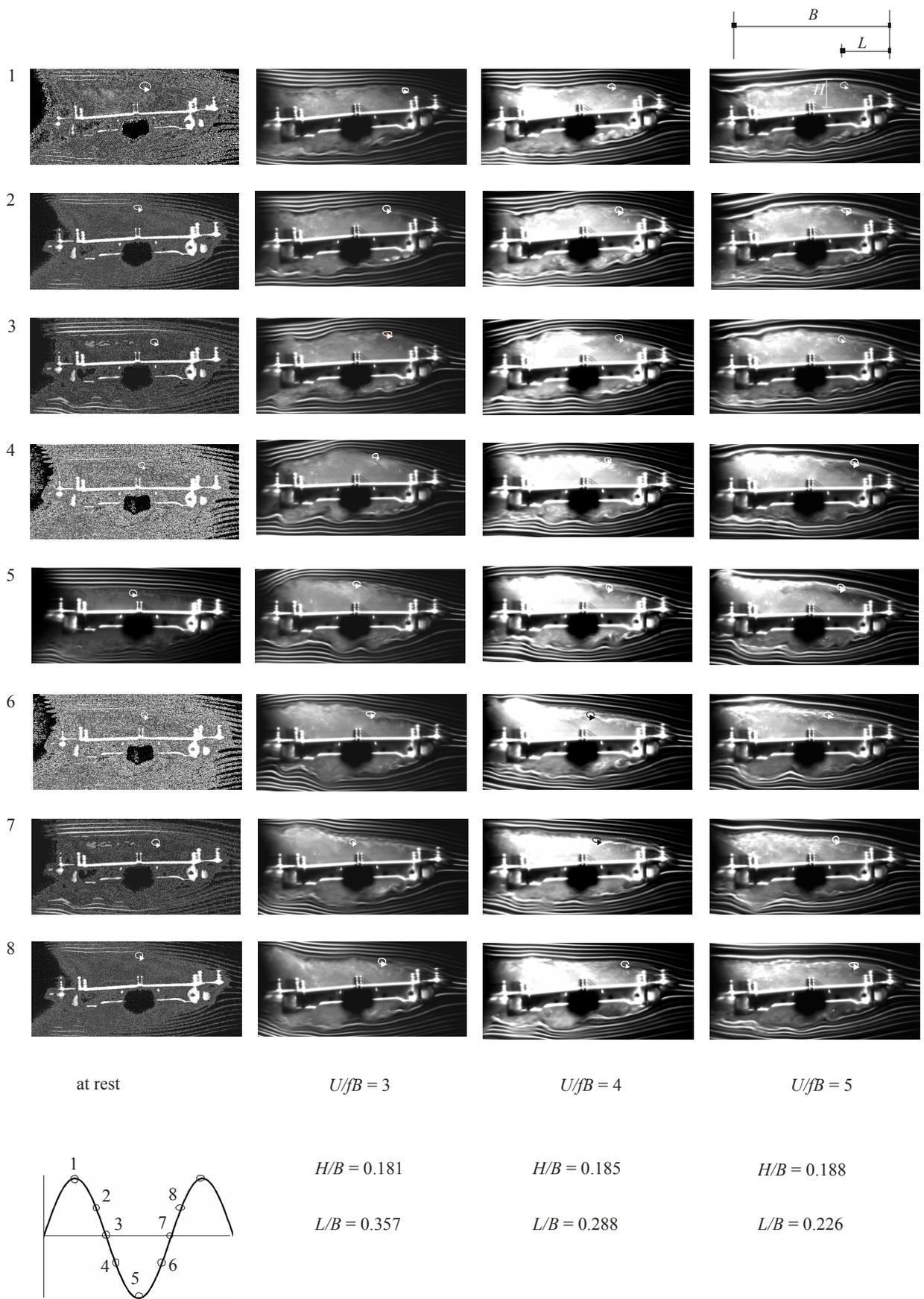
Figure 6 Instantaneous flows around the model without fairing (WOF)
