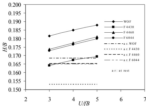
Figure 8 Ratio  $H/B$  to reduced wind velocity
