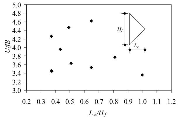
Figure 5(b) Flutter speed v.s. Ratio of the width of fairing tip to the depth of fairing
