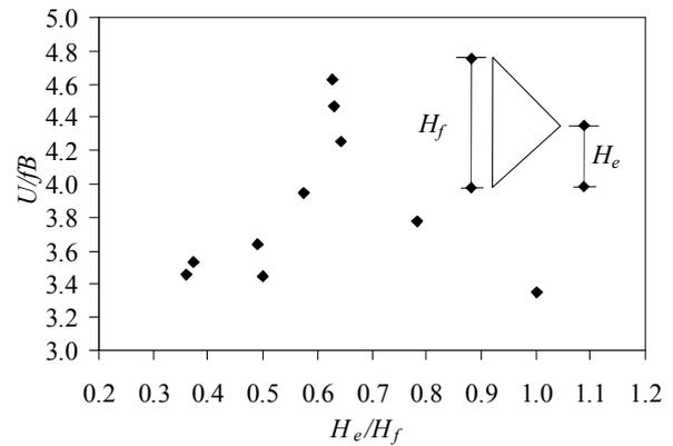
Figure 5(a) Flutter speed v.s. Ratio of the height of fairing tip to the depth of fairing
