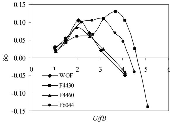
Figure 3 Aerodynamic damping ( $2\phi=2^\circ$ ,  $\alpha=3^\circ$ )
