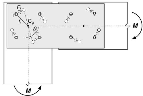
Fig.1 Example of moment-resisting connection
