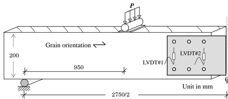
Fig.3 Simplified test set-up (half of symmetry)
