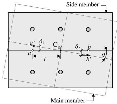
Fig.5 Schematic to measure the rotation of joint
