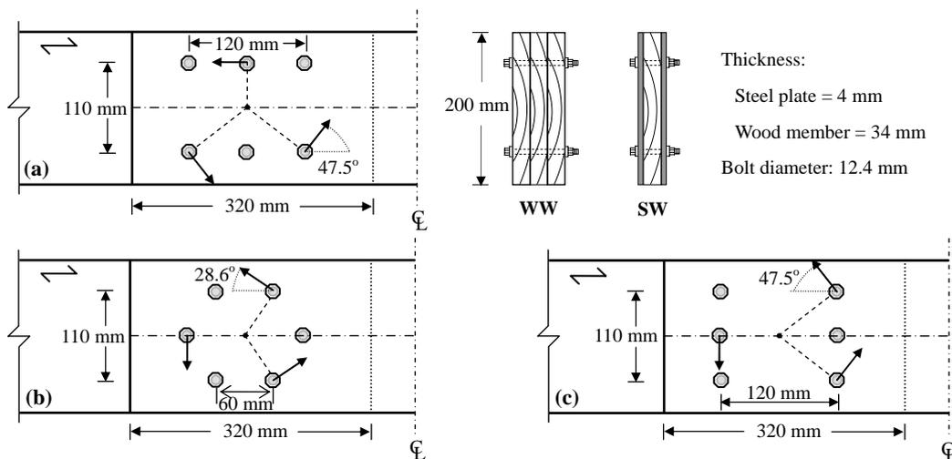
Fig.4 Fastener arrangements: (a) 6H bolt arrangement; (b) 6C bolt arrangement; and (c) 6V bolt arrangement
