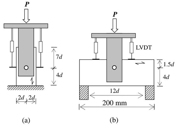
Fig.6 Single bolt connection test setup: (a) loading parallel to the wood grain; and (b) loading perpendicular to the wood grain.  $d$  is bolt diameter
