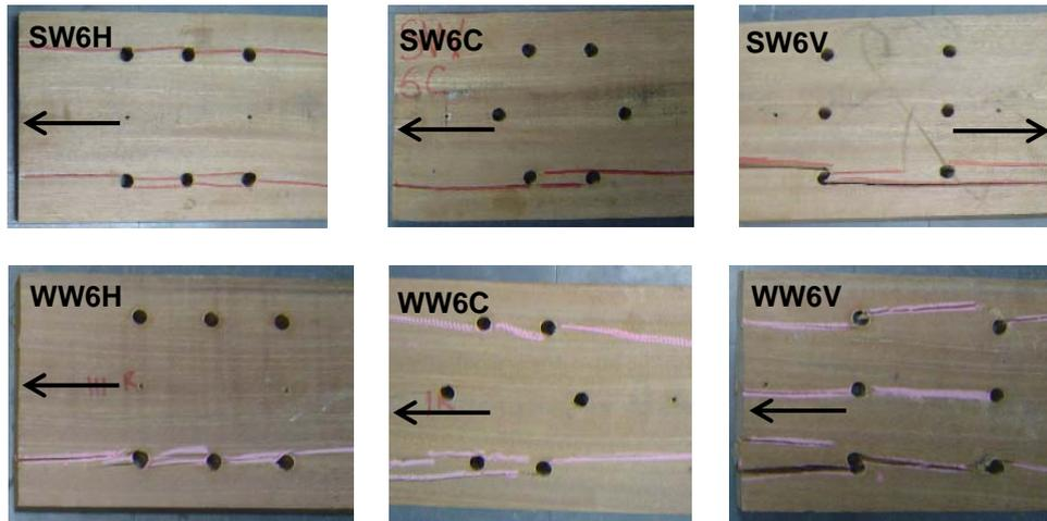
Fig.10 Splitting failure of wood main member (→: End member direction)
