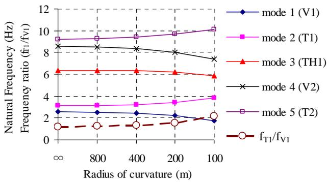
**Fig. 7** Natural frequencies/frequency ratios with varying of curvatures
