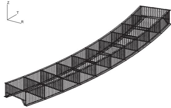
**Fig. 8** Typical full-height diaphragm model ( $R=200$ )
