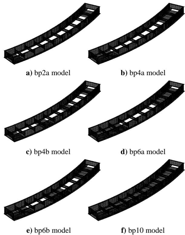
**Fig.10** Bottom-plate configurations ( $R=100m$ )
