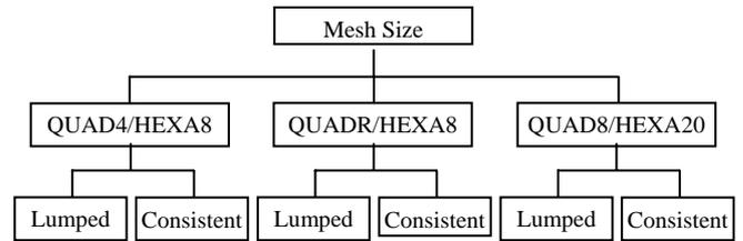
**Fig. 3** Flow chart of convergent test procedures
