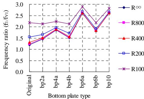
Fig. 12 Frequency ratios of bottom plate models
