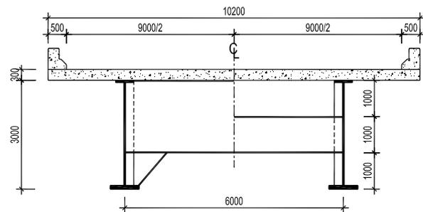
**Fig. 1** Cross section of the original bridge (mm)
