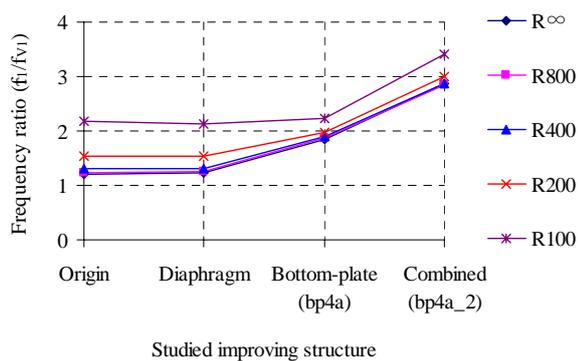
Fig. 15 Frequency ratios of studied improving structures
