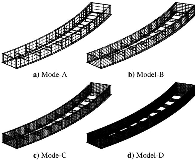
**Fig. 2** Four different mesh sizes (bridge deck is not shown)
