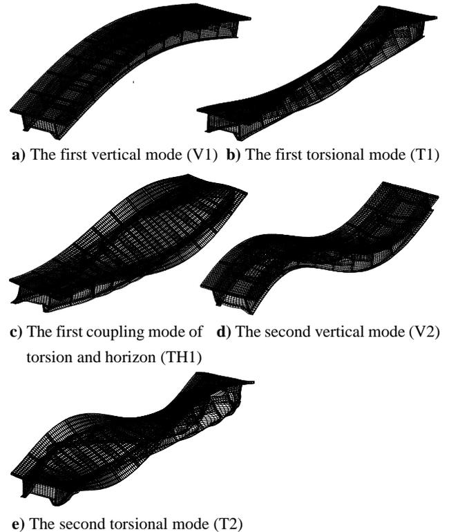
**Fig. 6** The first five mode shapes of the straight model
