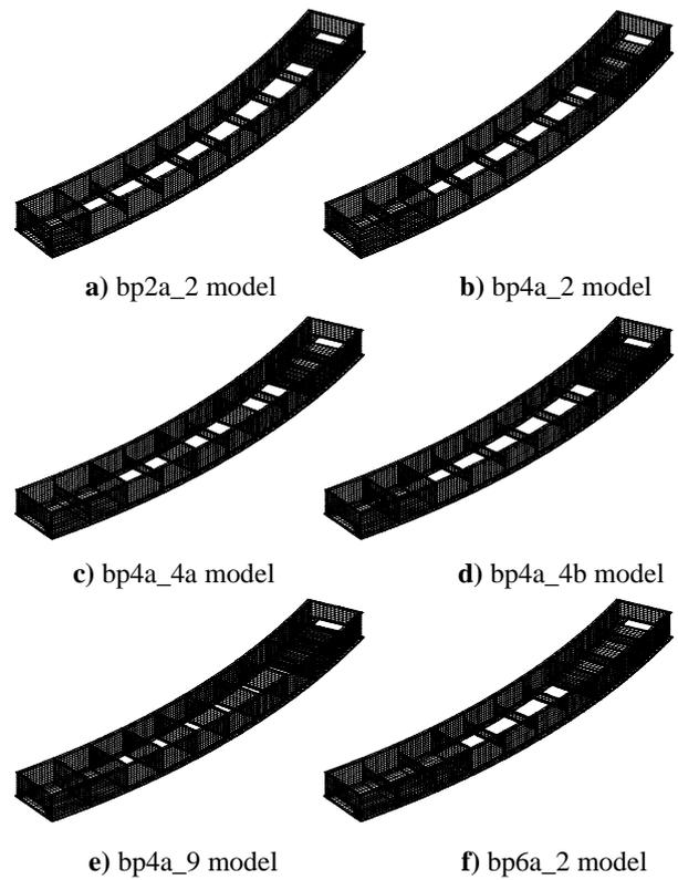
Fig. 13 Typical end stiffening configurations ( $R = 100m$ )
