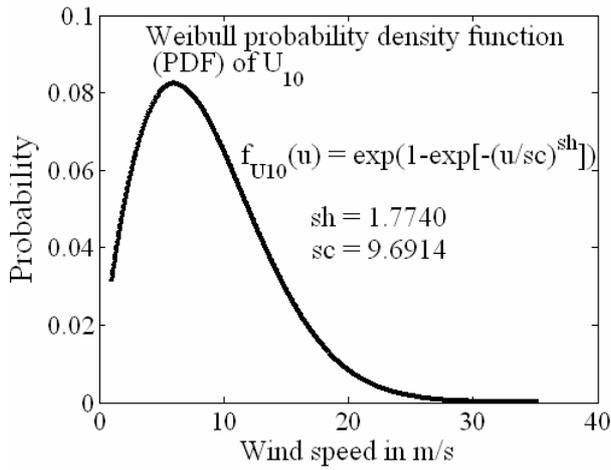
Fig.4 Probability density function of 10-minute wind speeds
