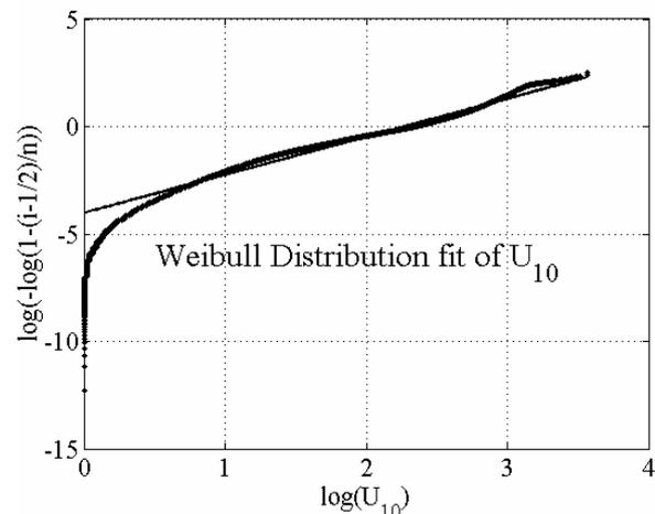
Fig.3 Cumulative density function of 10-minute wind speeds
