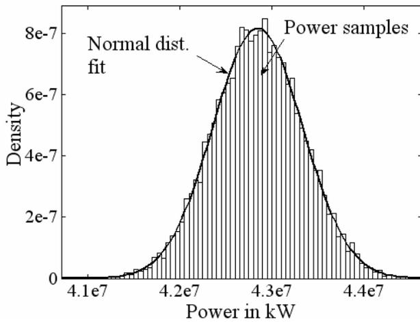
Fig.5 The pdf of the power output of a single wind turbine
