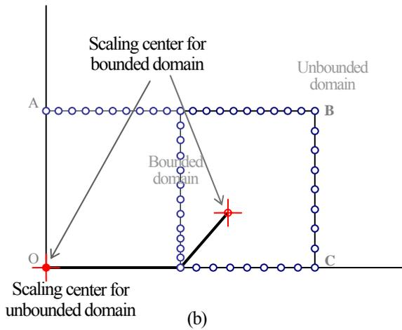
Fig. 6. a) Schematic diagrams and b) analytical model of double symmetric branched crack problem
