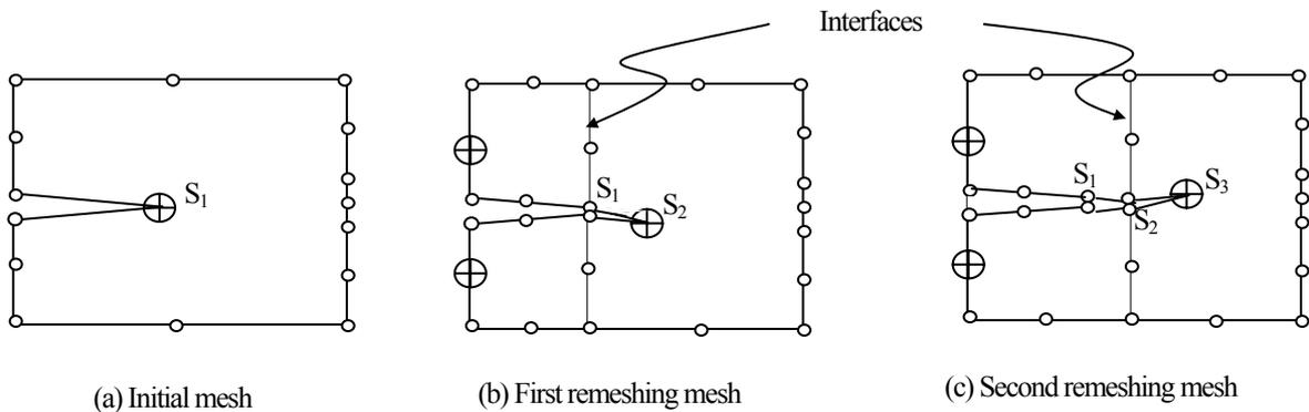
Fig. 3. The proposed remeshing procedure for crack propagation simulation ( $S_i$  &  $S_{i+1}$  are the old and new crack-tip)
