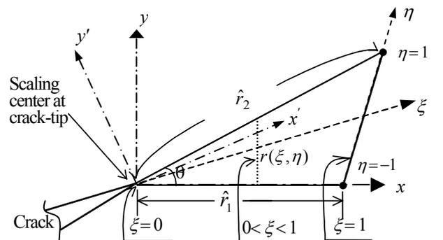
Fig. 2. SBFEM element with different coordinates
