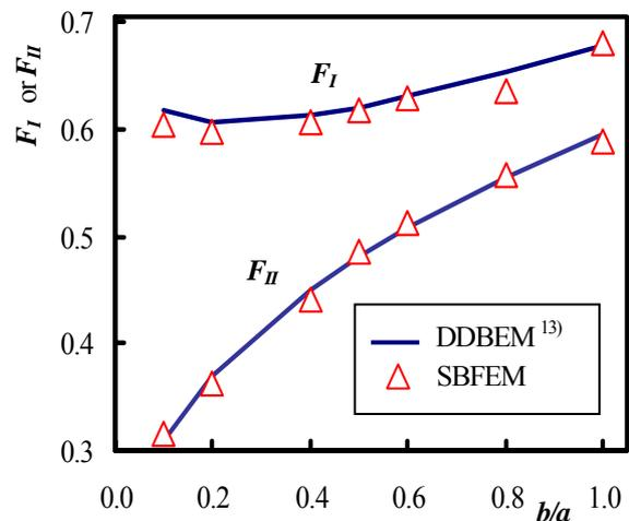
Fig. 7 Comparison of normalized SIFs at tips of branched crack for DSBC
