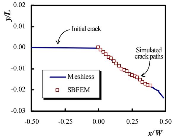
Fig. 9. Comparison of crack propagation trajectory.
