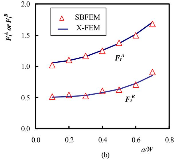
Fig 5. a) An analytical model of symmetric branched crack problem b) Comparison of computed normalized SIFs at crack tips A and B.
