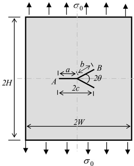
Fig. 4. Schematic diagrams of symmetric branched crack problem
